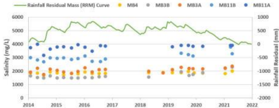
Figure 3-3 Groundwater Salinity (Total Dissolved Solids) Over Time vs RRM (deviation from mean monthly rainfall plotted against time)
